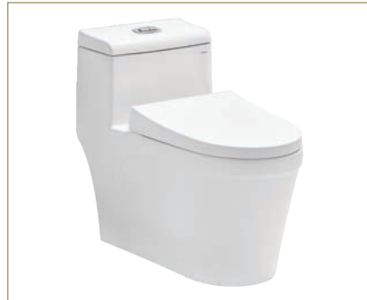
Sean one piece EWC S Soft close duroplast seat cover & fittings Syphonic flushing for more effective cleaning Anti-microbial nano glaze for superior sheen & hygiene Swirl flush for superior cleaning 300 mm WD 730 x 395 x 660 mm Cat. No. A1014102 ₹ 25000
